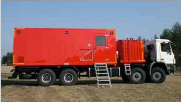
Truck Mounted Unit with 6.000 l Diesel Tank
