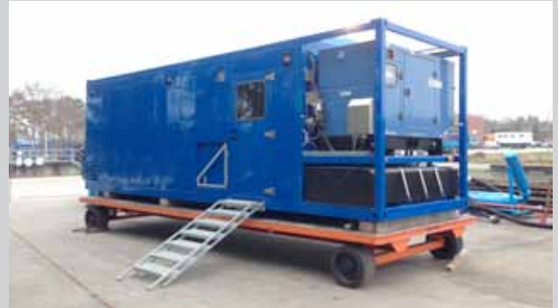
Skid Mounted System powered by Generator
